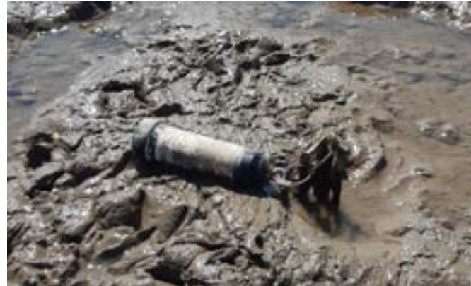
B4+ mini buoys measuring wave orbital movements – informing hydrodynamics
