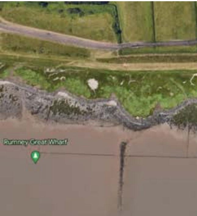
Photo 1: Rhymney wharf flood embankment post 3 January 2014 tidal event (8.03m above Ordnance Datum at Newport 2 gauge)
